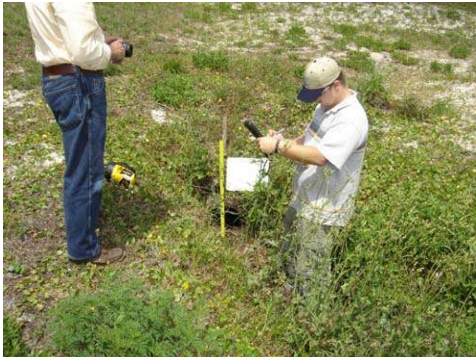
Figure 4 Project Manager Jason Baum (r) measures outfall pipe in Panama City off of Beach Drive, while Lyman Barger (l) enters location data into GPS unit. Bay County, Florida . Protocols were developed as a training program for BEST/FSAB volunteers.
